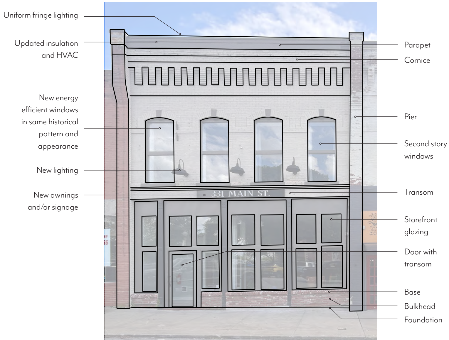
Figure 2.28: Prototype Facade Features
